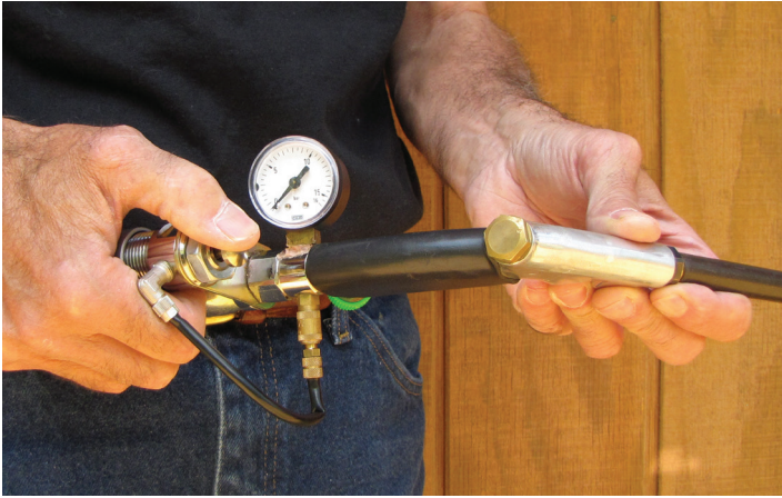
Fig. 17.5. Adjustable, CO 2 -powered blow pipes can be used to dart all species of furbearers weighing >3 kg (6.6 lb); holographic sights greatly increase the ability of the user to accurately place the darts.
