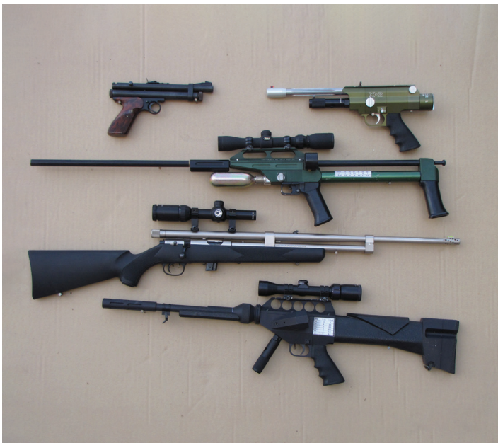
Fig. 17.6. Examples of dart guns, including from top left: Cap-Chur Short Range Projector (CO 2 powered), Pneu-Dart X-2 (CO 2 powered), Dan-Inject (CO 2 powered), Pneu-Dart model 389 (.22 caliber-blank powered), and Pneu-Dart X-Caliber (CO 2 powered).
